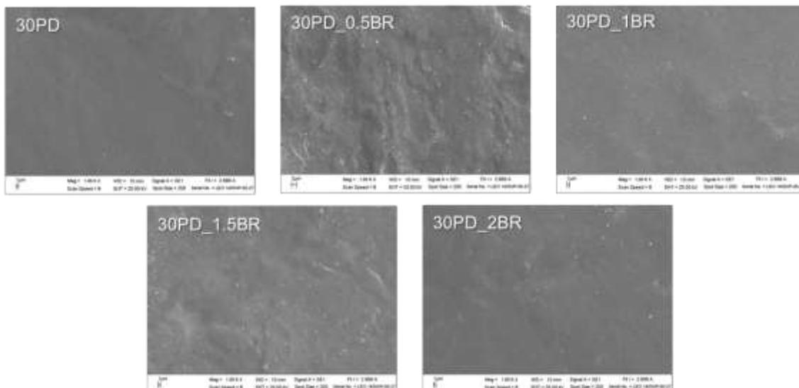
**Figure 1.** Surface morphology of the CBFS without cross-linker (30PD), cross-linked CBFS (30PD\_0.5BR, 30PD\_1BR, 30PD\_1.5BR and 30PD\_2BR)
