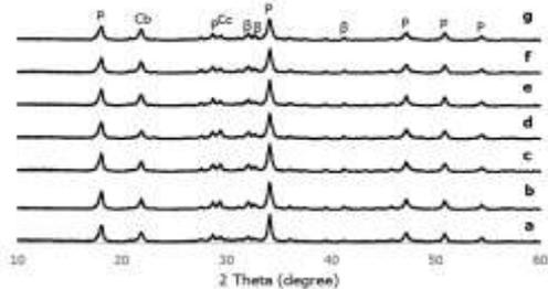
**Figure 8.** The XRD pattern of cement paste hydrated for 28 days: (a) without activator, (b) with 1%  $\text{Na}_2\text{SiO}_3$ , (c) with 2%  $\text{Na}_2\text{SiO}_3$ , (d) with 3%  $\text{Na}_2\text{SiO}_3$ , (e) with 1%  $\text{Na}_2\text{CO}_3$ , (f) with 2%  $\text{Na}_2\text{CO}_3$  and (g) with 3%  $\text{Na}_2\text{CO}_3$ .
