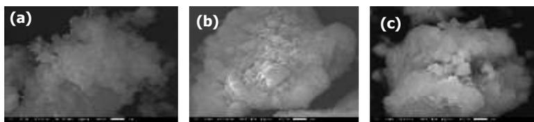
**Figure 5.** SEM micrographs of hydrated cements for 7 days: (a) without activator, (b) 3%  $\text{Na}_2\text{SiO}_3$  and (c) 3%  $\text{Na}_2\text{CO}_3$ .
