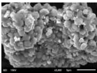
**Figure 3.** Scanning electron micrographs of dicalcium silicate from BRHA.
