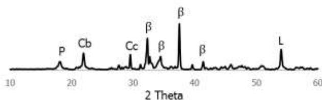
**Figure 4.** The XRD pattern of dicalcium silicate. (P = Portlandite, Cc = Calcite, Cb = Cristobalite ( $\text{SiO}_2$ ),  $\beta$  = Lanite ( $\text{Ca}_2\text{SiO}_4$ ), L = Lime ( $\text{CaO}$ )).
