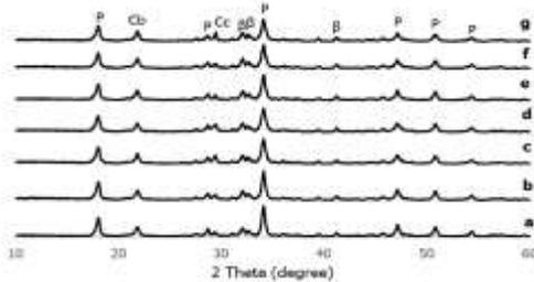
**Figure 7.** The XRD pattern of cement paste hydrated for 7 days: (a) without activator, (b) with 1%  $\text{Na}_2\text{SiO}_3$ , (c) with 2%  $\text{Na}_2\text{SiO}_3$ , (d) with 3%  $\text{Na}_2\text{SiO}_3$ , (e) with 1%  $\text{Na}_2\text{CO}_3$ , (f) with 2%  $\text{Na}_2\text{CO}_3$  and (g) with 3%  $\text{Na}_2\text{CO}_3$ . (P = Portlandite,  $\beta$  = Lanite ( $\text{Ca}_2\text{SiO}_4$ ), Cc = Calcite, Cb = Critobalite
