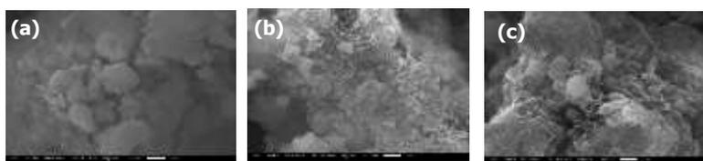
**Figure 6.** SEM micrographs of hydrated cements for 28 days: (a) without activator, (b) 3%  $\text{Na}_2\text{SiO}_3$  and (c) 3%  $\text{Na}_2\text{CO}_3$ .
