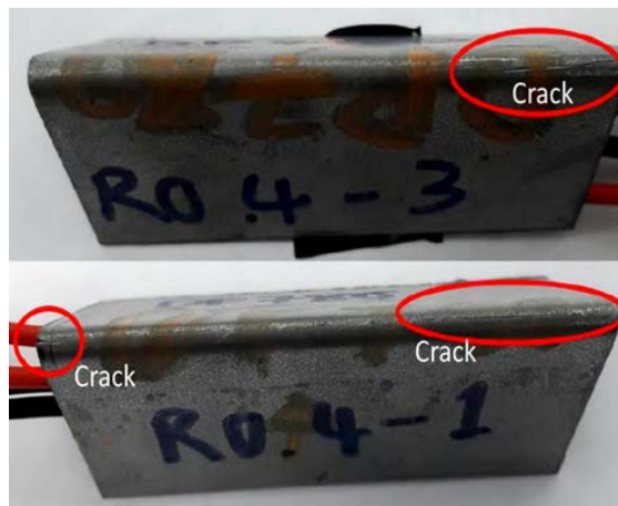
Figure 6. Example of cracks on the testpiece
